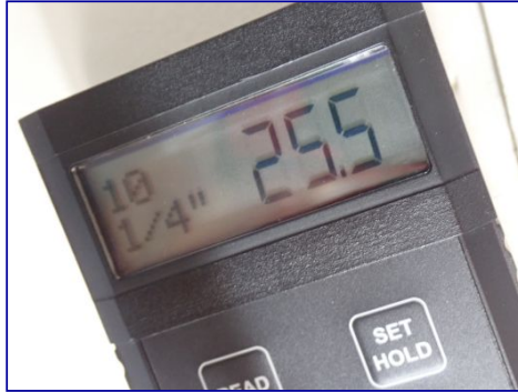
Moisture evident. Hall bathroom next to exhaust vent.
