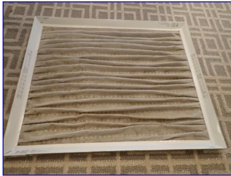
Air filter dirty. Loft HVAC closet.
