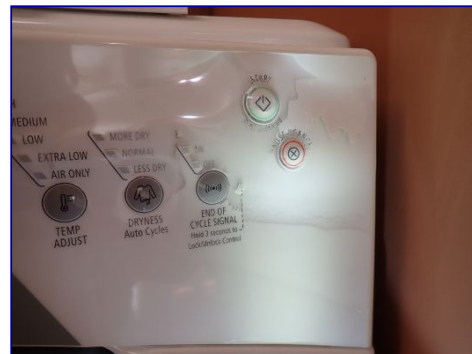
Control panel damaged. Delaminating.
