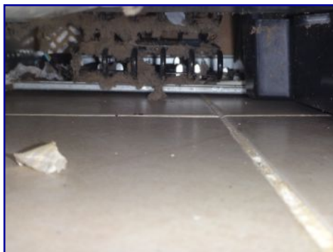
Coils dirty. Refrigerator bottom rear.
