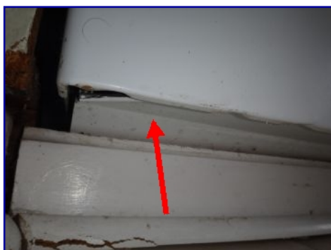
Dishwasher damaged. Bottom panel bent and loose.
