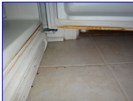
Refrigerator damaged. Rust visible.
